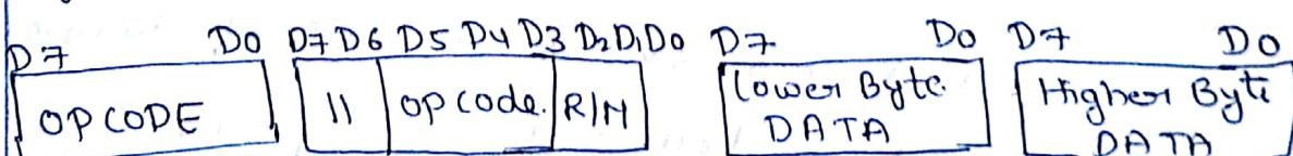
6. Immediate operand to memory with 16-Bit Displacement.
